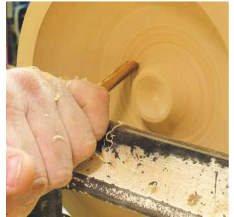
▲ Pic.12 The same tool is used here working from the inside to the bottom of the curve – don't come up the side because that could lead to a dig in. It's a bit like doing a cove on spindle work
